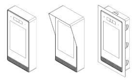
Surface mount, surface mount with hood and flush mount. A back box <u>must be used</u> to obtain IP65 rating.
